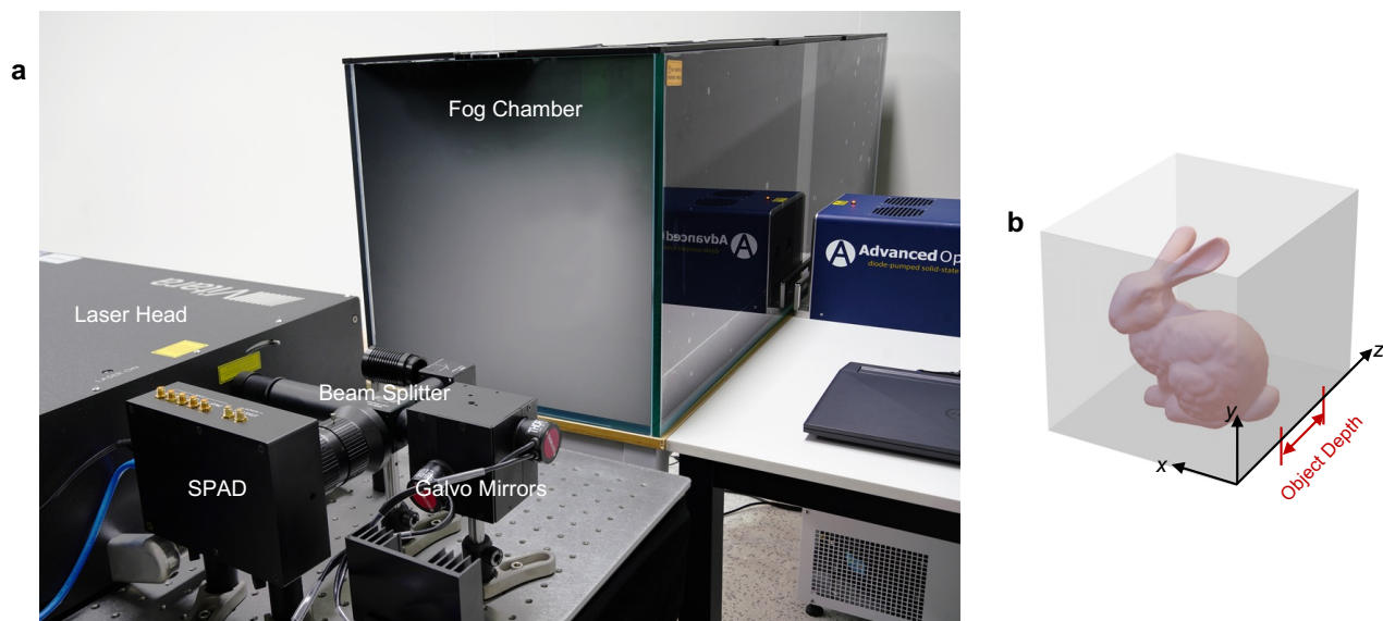
Supplementary Fig. 3 Photograph and layout of the fog scattering scenario. a An artificial fog chamber with a size of 50cm × 50cm × 150cm provides the dynamic scattering environment. b The object is embedded in the fog and its depth range is defined as the distance range from the front surface of the scattering media to the object.
