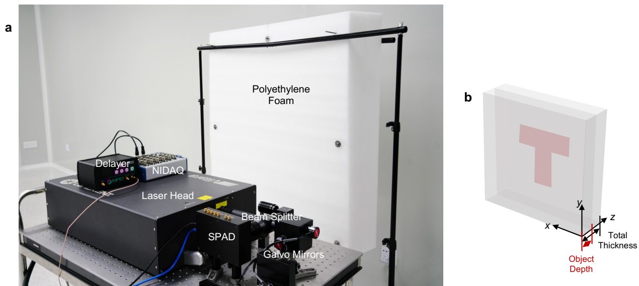
Supplementary Fig. 2 Photograph and layout of the polyethylene foam scattering scenario. a Confocal imaging system captures the photons reflected from the foam scenario. b The total thicknesses of the foam range from 12cm to 25cm. The object is embedded in the foam and its depth is defined as the distance from the front surface of the scattering media to the object.
